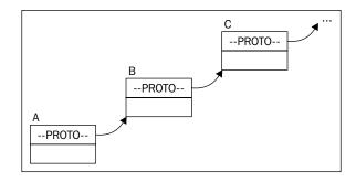
In this illustration, an object A contains a number of properties. One of the properties is the hidden \_\_proto\_\_ property, which points to another object, B. B's \_\_proto\_\_ property points to C. This chain ends with the Object.prototype object - the grandparent, and every object inherits from it.
